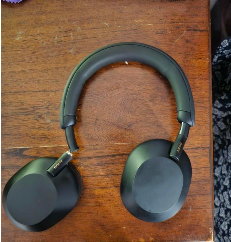
Figure 1: Fully Detached Swiveling Hinge Due to Defect. 1
