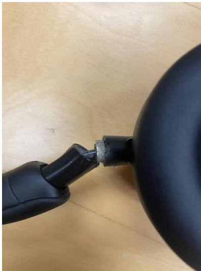
Figure 1: Plaintiff Kanter's Headphones with manifestation of Defect.
