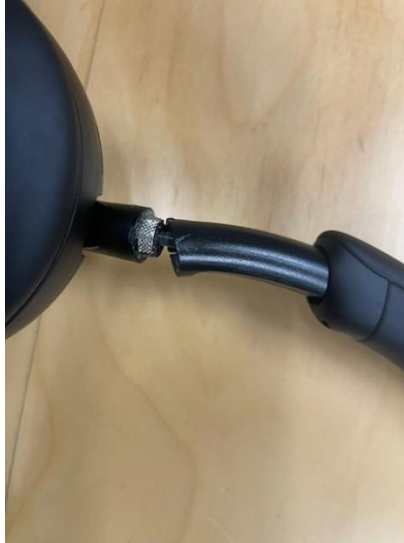
Figure 2: Plaintiff Kanter's Headphones with the Defect showing separation between the headband and ear cup.
