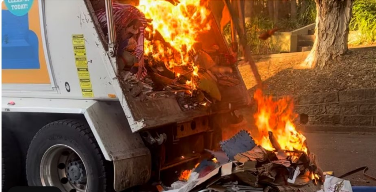
Figure 3 - A fire in a truck caused by a Lithium-ion battery 12
