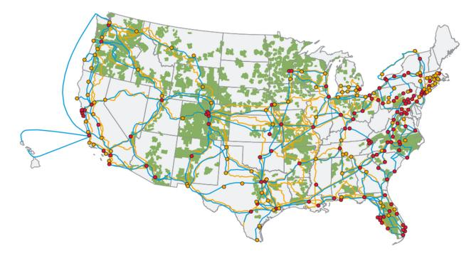
In this map, the shaded green areas represent local territories serviced by traditional copper wire cable lines whereas the orange and blue lines represent the fiber optic cable lines owned by CenturyLink and Level 3, respectively.
