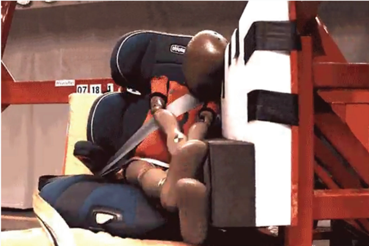
The dummy in the Chicco KidFit did make head impact with the door during our crash testing, though overall the seat scored well. Video: Calspan
