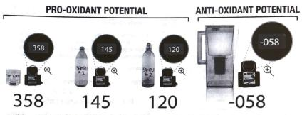
If the number value displayed by the ORP meter is positive (above zero) then the water has oxidizing potential. If the number's negative (below zero) then the water has antioxidant potential.
