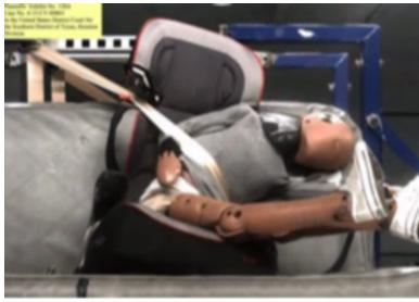
54. Direct testing comparisons show that the Big Kid Booster models with side wings performed no better in side-impact testing than Big Kid Booster models without side wings:
