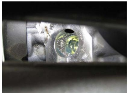
59. By March 2011, Bosch was continuing to receive "a respectable number of claimed [failures in] CR-pumps Typ CP4 for US-07" about which Volkswagen dealerships were reporting "[m]etal particle[s] at the filter.' In a few cases the [dealer] use[s] this as an indication,
