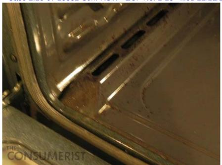
The attached photos show the interior of the oven, which went from clean/new to this after cooking 1 time at a high temperature (chicken) – and AFTER 2 cleaning cycles.
