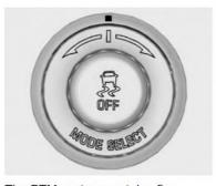
The PTM system contains five modes. These modes are selected by turning the Selective Ride Control/Performance Traction Management MODE SELECT knob on the center console. Scroll up or down through modes 1–5 by turning the MODE SELECT knob to the right or left.
