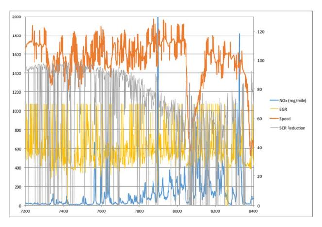
178. The same behavior is observed in the plot below. Emissions are 63 mg/mile for about 400 seconds before the SCR system is de-rated (i.e. urea injection is reduced). After the SCR system is de-rated, emissions increase to 167 mg/mile.
