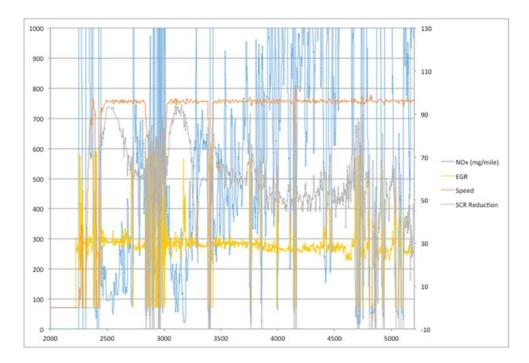
233. Another instance in the following plot, where the reduction in SCR effectiveness begins to reduce at 2,900 seconds. The SCR effectiveness reduces from well over 90% to approximately 50%, just as before, with a composite NOx emission rate of 428 mg/mile. Prior to the reduction in urea injection, the emission rate is 58 mg/mile, well below the standard. After the reduction in urea injection, the emission rate increases to 586 mg/mile.
