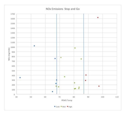
237. Similarly, for steady highway conditions on flat roads, the average NOx emission rate is 615 mg/mile, or 3 times the standard of 200 mg/mile. We observe emission rates as high as 1,254 mg/mile, or 6.3 times the standard. On average, the SCR effectiveness is reduced from 86% in cases where the vehicle meets the standard to 54% in cases where the vehicle exceeds the standard.
