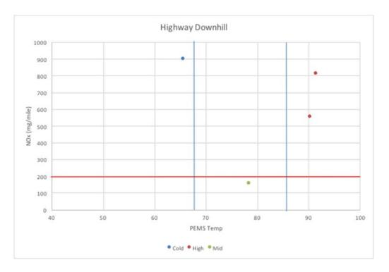
242. It is thus clear that the vehicle is able to detect both uphill and downhill grades and reduce the level of urea injection. This defeat device results in a reduced effectiveness of the SCR and EGR systems and dramatic and consistent increases in NOx above the standard. Combined with the timeout defeat device that reduces the SCR effectiveness after a short period of time, the vehicle rarely meets the NOx emission standard.
