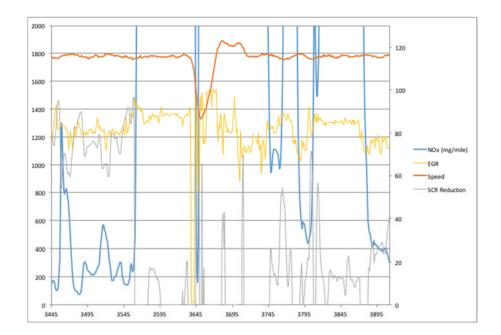
208. Here we see a plot where the SCR system is de-rated on a periodic basis (gray line) over the course of 1.2 hours, driving the NOx up to levels above 200 mg/mile. As a result, the overall NOx emission rate for this segment is 131 mg/mile.
