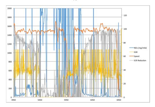
176. The following plot shows similar behavior. At around 16,150 seconds, the SCR system reduction begins to decrease and NOx begins to increase. At 16,350 seconds, the EGR system is shut off completely and the SCR reduction goes to near 0. Again, the NOx emissions (blue line) increase to values that exceed the maximum 2,000 mg/mile limit on the chart. These changes are not associated with any load change due to speed or road grade.
