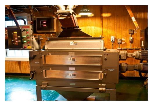
62. As the photo depicts, the mill is powered by two electronically driven motors and the entire mechanized and/or automated process is controlled by a set of electronic control panels as seen to left of the machine. *See*,  $\P$  61.
