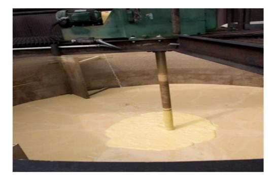
66. As the picture above indicates, the grain mash and other ingredients are mixed using a machine. More specifically, a paddle like device, which is attached to an electronic motor, is used to blend the mixture. The motor is mounted onto metal beams that rest above the vat into which the mixture sits. This mixing process is mechanized, automated, and involves little to no human supervision, assistance or involvement; thus, it is clearly not "Handmade" as Defendants advertise.
