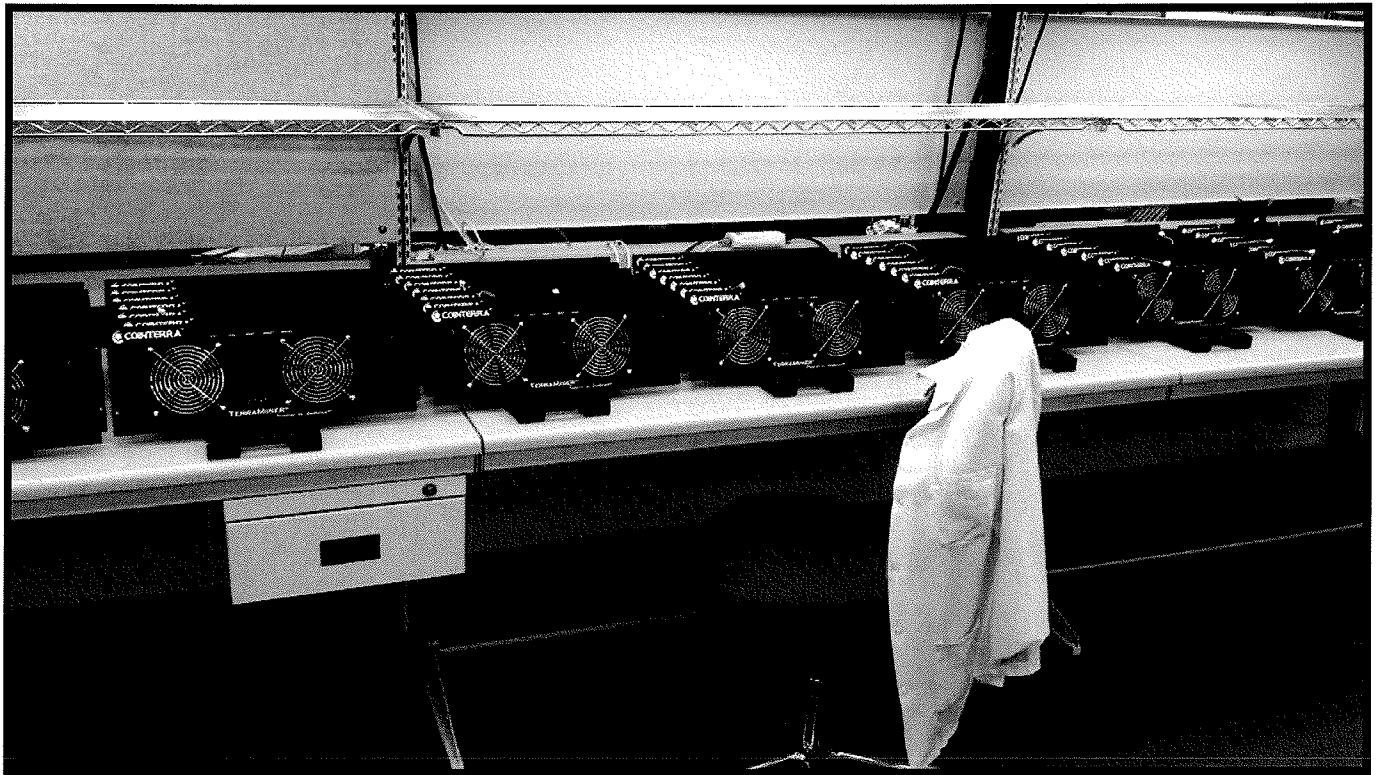
TerraMiner front panels (populated with fans and grills) racked and ready to be bolted onto the chassis
